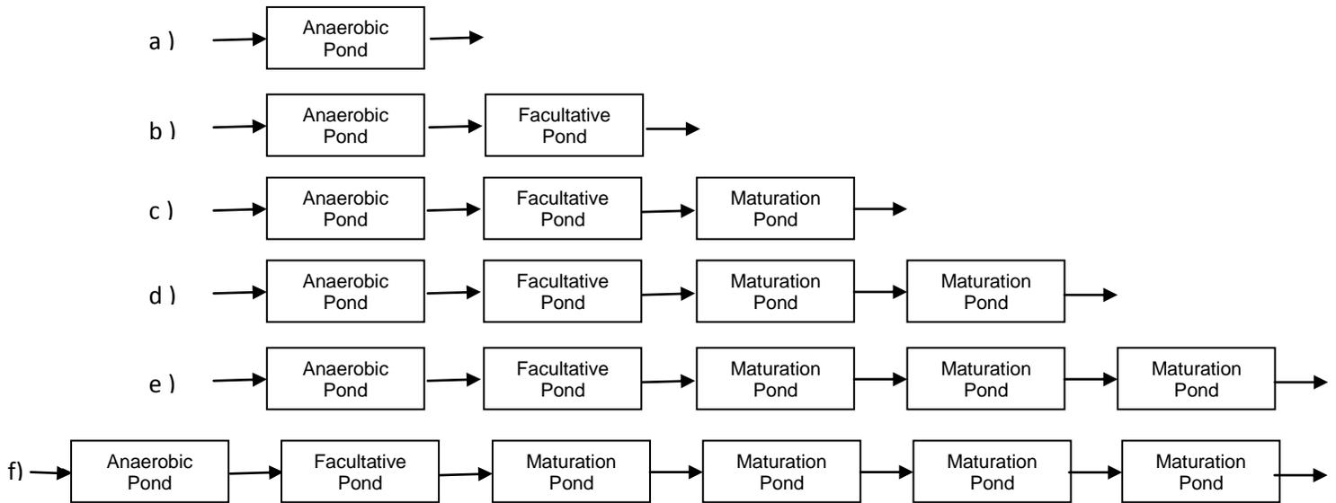
Figure 1: different alternative of waste stabilization ponds used for treatment of wastewater
