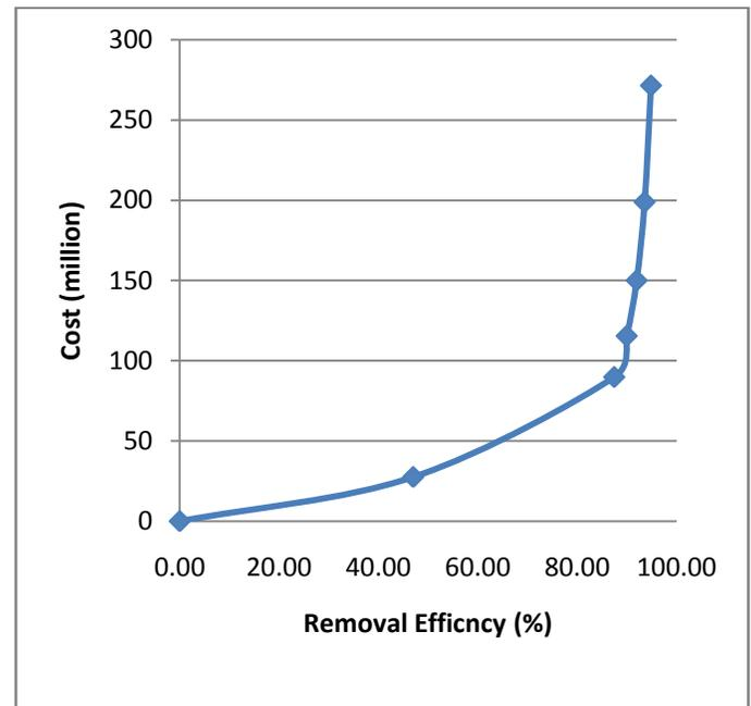
Figure 2. Relationship between cost and removal efficiency in terms of BOD removal
