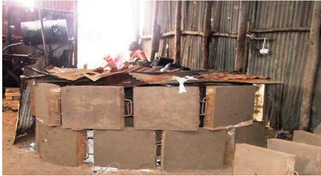
Fig 3: Moulds baked using charcoal at one of the foundries
