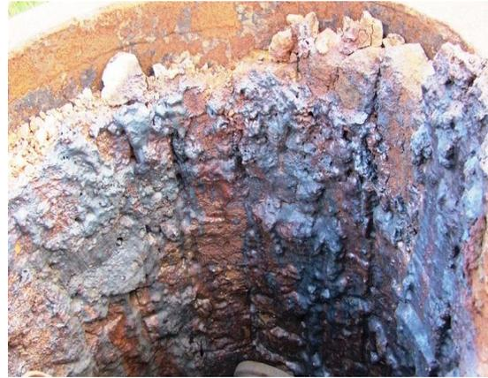
**Fig 7:** Left is a worn furnace cover lining and on the right a worn wall lining as evidenced concerning poor maintenance weaknesses in Ugandan foundries
