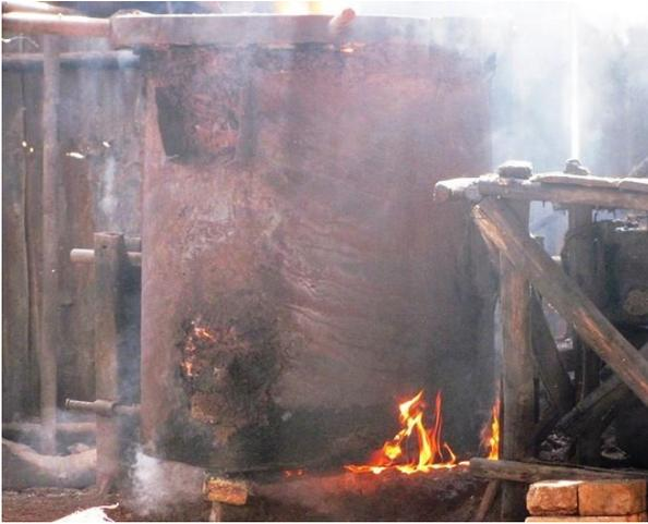
**Fig 8:** A crucible furnace in operation with fire coming from the bottom
