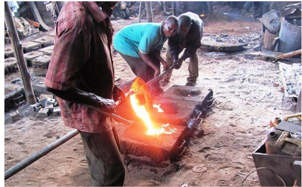
**Fig 9:** Foundry workers pouring molten metal from the ladle to the moulds while it spills on the sides
