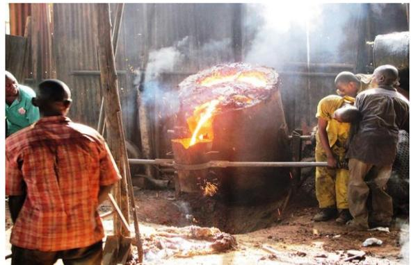
**Fig 2:** A tilt furnace in operation at one of the foundries visited
