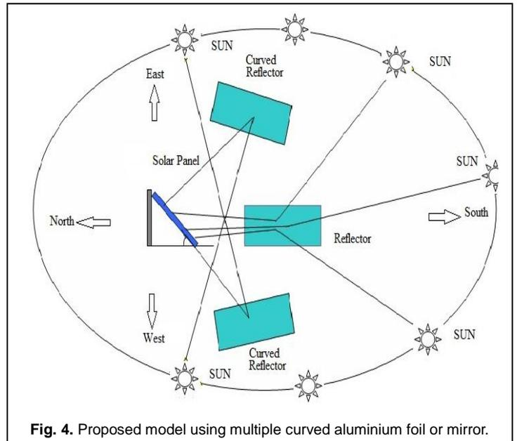
Fig. 4. Proposed model using multiple curved aluminium foil or mirror.
