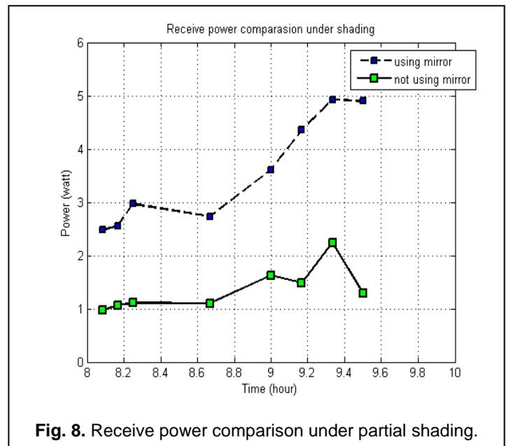
**Fig. 8.** Receive power comparison under partial shading.
