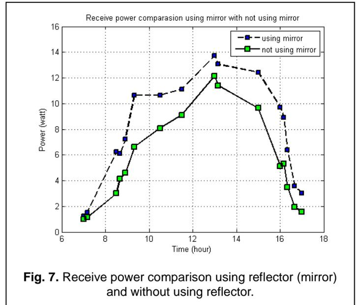
**Fig. 7.** Receive power comparison using reflector (mirror) and without using reflector.
