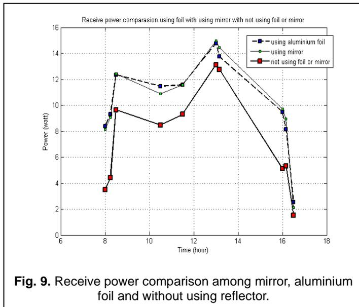
**Fig. 9.** Receive power comparison among mirror, aluminium foil and without using reflector.
