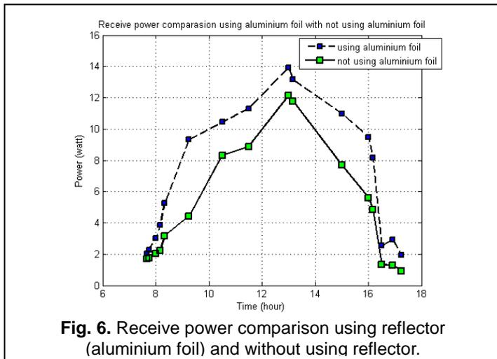
**Fig. 6.** Receive power comparison using reflector (aluminium foil) and without using reflector.
