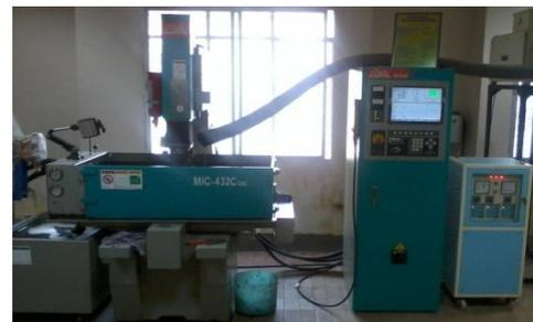
Fig.3 ECOWIN MIC-432C EDM
