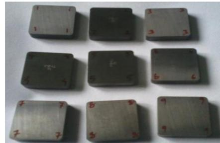
Fig .2 Tungsten Carbide Plates
