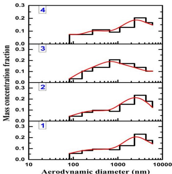
**Fig. 2.** Average mass size distribution of aerosol particles in the selected four points in El-Minia city.
