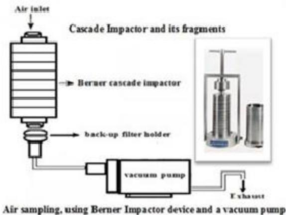
**Fig 1.** Aerosol sampling set-up using Berner Low pressure cascade impactor (BLPI)
