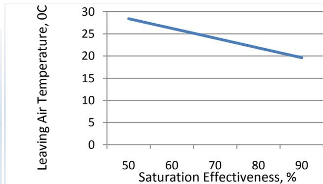
**Figure 3.0** Leaving Air Temp. Vs Saturation Effectiveness
