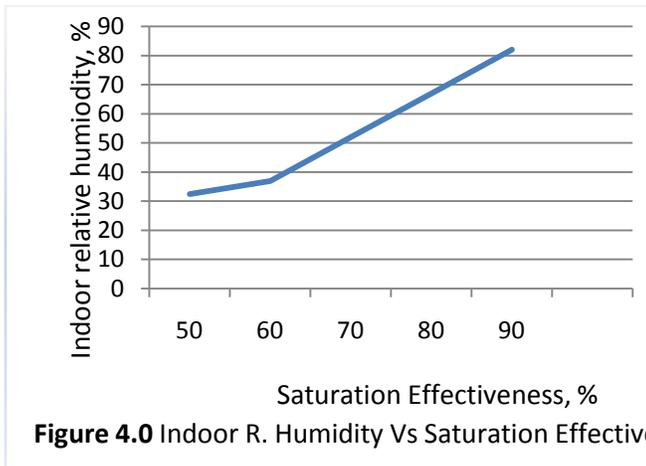
**Figure 4.0** Indoor R. Humidity Vs Saturation Effectiveness
