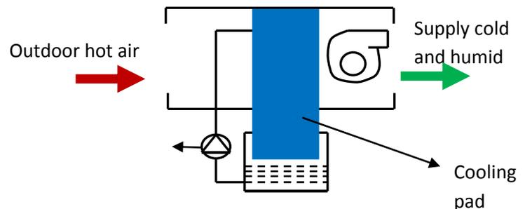
Figure 1.0 Direct Evaporative Cooler
