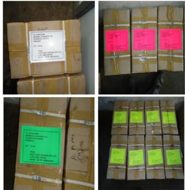
**Fig. 10.** Marking and Standardization of the Templates with different color codes. (each color code specifies a particular company/product which helps in minimizing the problem of dispatching the different product to other company).
