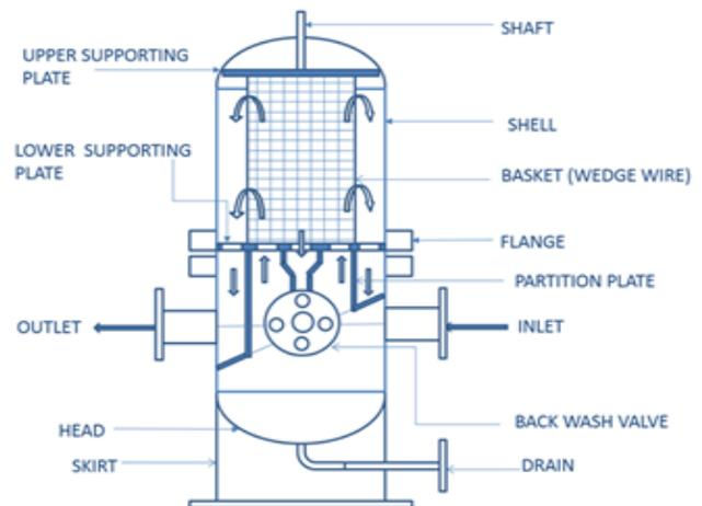
**Fig1:** Self Cleaning strainer ( AutoCAD Generated)
