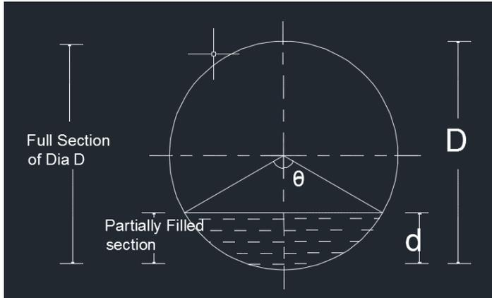
**Figure 2.** Sewer pipe line cross section
