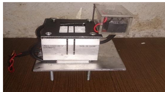
Figure 9. Prototype TEG (Thermal electric Generator) Small Modular
