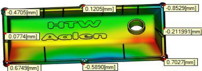
Fig. 16. Deflection in All Direction for Inside Created Mold
