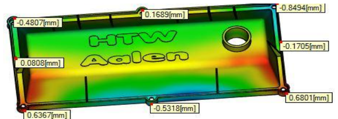
Fig. 13. Deflection in Y-Direction for Imported Mold
