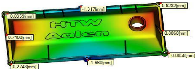
Fig. 15. Deflection in Z- Direction for Imported Mold
