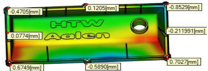
Fig. 12. Deflection in Y-Direction for Imported Mold
