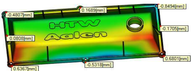
Fig. 17. Deflection in All Direction for Imported Mold
