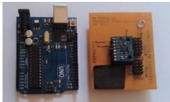
Figure 11. PCB of Arduino Based Flight Controller
