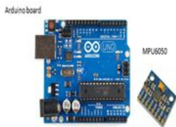
Figure 10. Arduino board and MPU 6050 sensor to build flight controller
