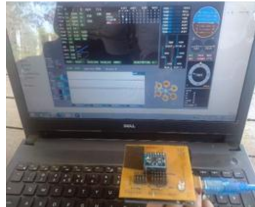
Figure 9. PID tuning with flight controller by the help of GUI before flying
