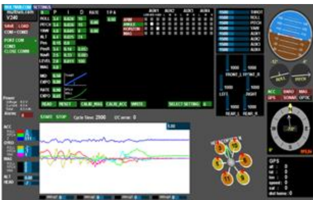
Figure 8. Hexacopter tuning GUI written in visual basic
