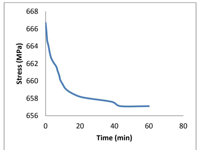
**Figure 2.3:** Stress Vs time graph for torsional load at twisting angle 45 degree
