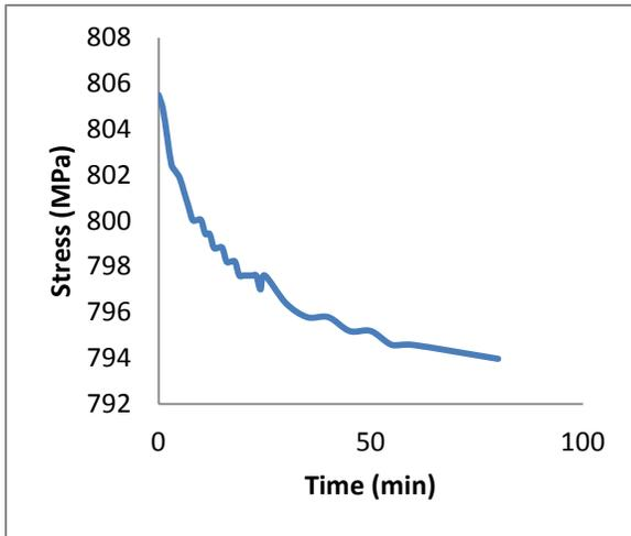
**Fig 1.2:** Stress Vs time for SMA rod under bending load at constant strain
