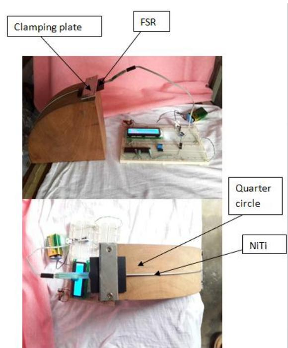
Figure 1.1: images of bending stress relaxation test
