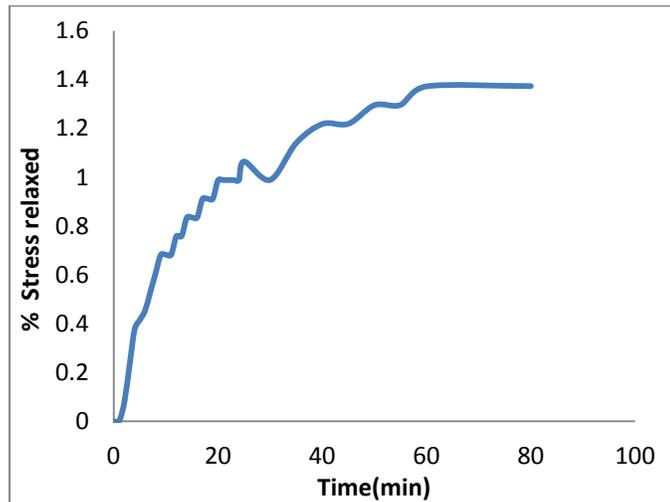
**Figure 1.3:** % stress relaxation Vs time for SMA rod under bending load
