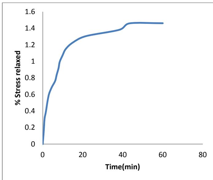
**Figure 2.4:** % stress relaxed Vs time of SMA rod for torsional load at 45 degree twisting angle
