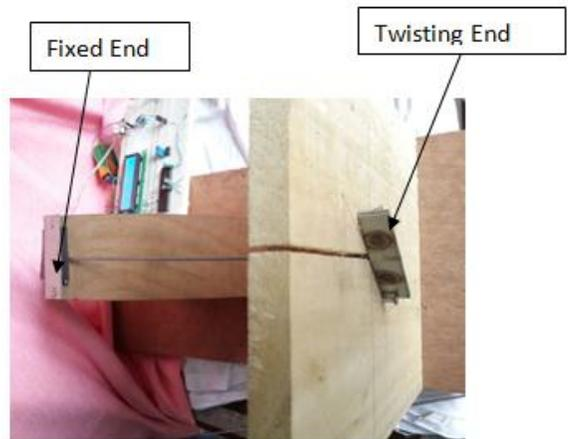
**Figure 2.1:** image of set up for torsional load
