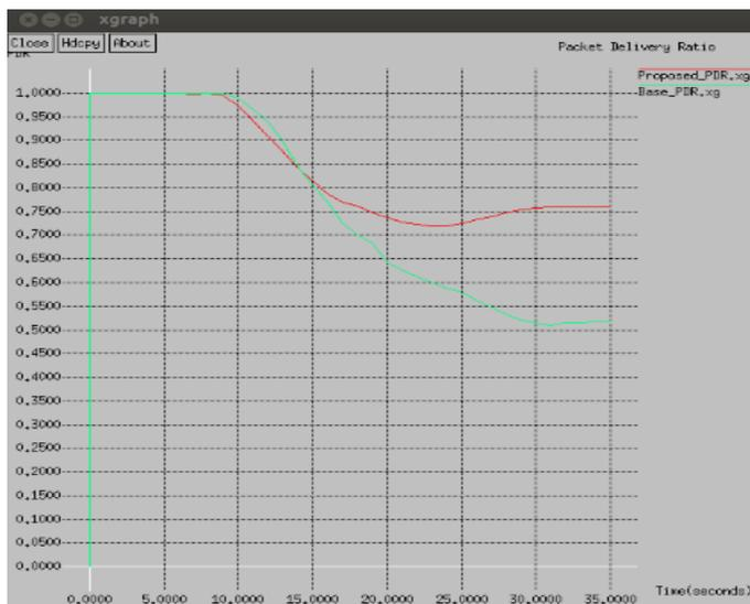
**Fig.2.** Comparison of packet delivery ratio (PDR) of modified EECPK-means approach – red to existing EECPK-means technique – green
