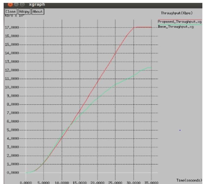
**Fig.4.** Comparison of throughput of proposed strategy – red to Existing EECPK-means technique – green
