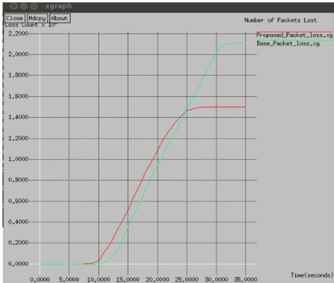
**Fig.5.** Comparison of number of packets lost of proposed strategy – red to existing EECPK-means technique - green
