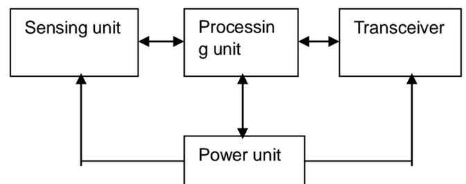
**Fig.1.**Basic Building Block of Sensor Node
