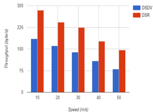
**Fig:** Variation in UDP throughput with an increase in mobility for Freeway Mobility Model.
