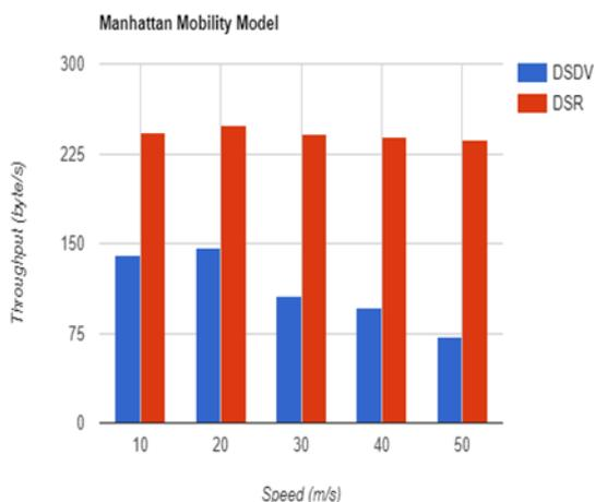
**Fig:** Variation in UDP throughput with increase in mobility for Manhattan Mobility model
