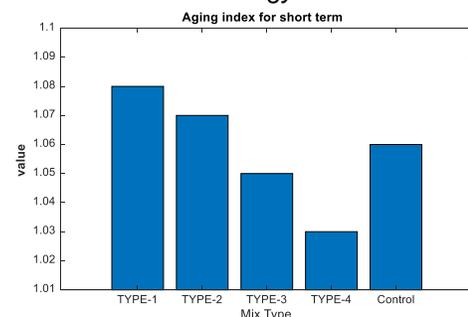
Figure 4: Aging index for control and asphalt mixtures
