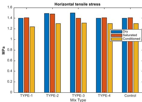
**Figure 5:** Horizontal tensile stress at center specimen
