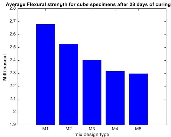
**Figure 10:** Comparison of average flexural tensile strength for concrete mix after 28 days
