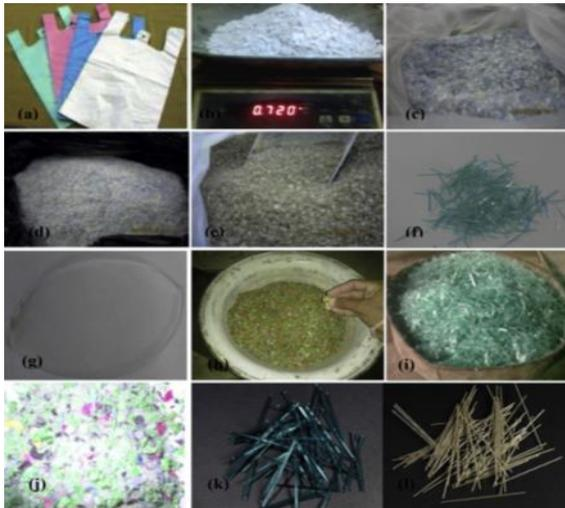
**Figure 2:** Different forms of waste plastic: (a) Polyethylene (b) Sample of waste plastic (c) PET-aggregates PC (d) PET aggregate PF (e) PET aggregate PP (f) Short laminar fiber (g) Sample of 'O' fiber (h) Shredded fiber (i) Hand Cut fiber (j) Granulated Plastic (k) polyethylene terephthalate and (l) polyethylene terephthalate [10]
