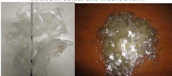
**Figure 4:** Polyethylene terephthalate (PET) waste cup before cutting and after cutting
