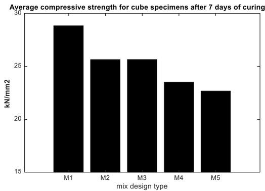
Figure 5: Comparison of average compressive strength for concrete mix after 7 days
