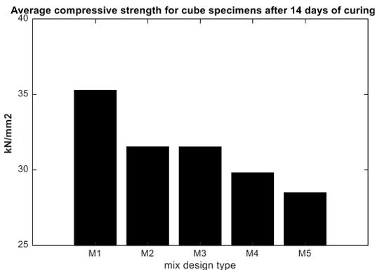
Figure 6: Comparison of average compressive strength for concrete mix after 14 days
