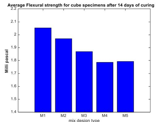
Figure 9: Comparison of average flexural tensile strength for concrete mix after 14 days
