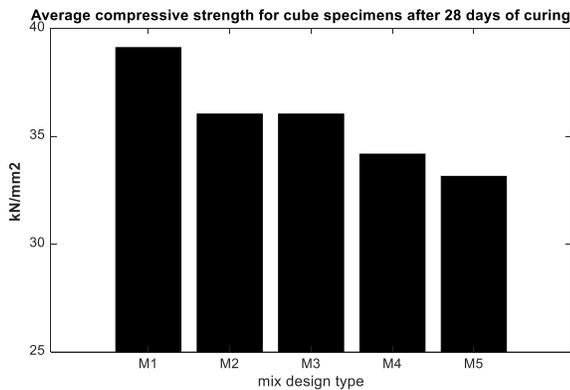
Figure 7: Comparison of average compressive strength for concrete mix after 28 days
