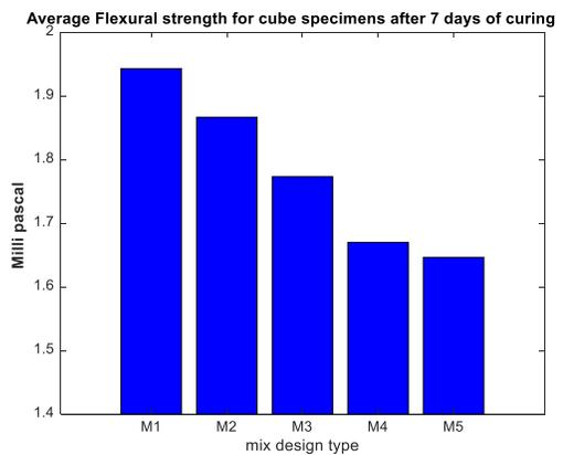
Figure 8: Comparison of average flexural tensile strength for concrete mix after 7 days
