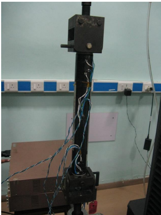
Fig. 4 The support tube under static load test
