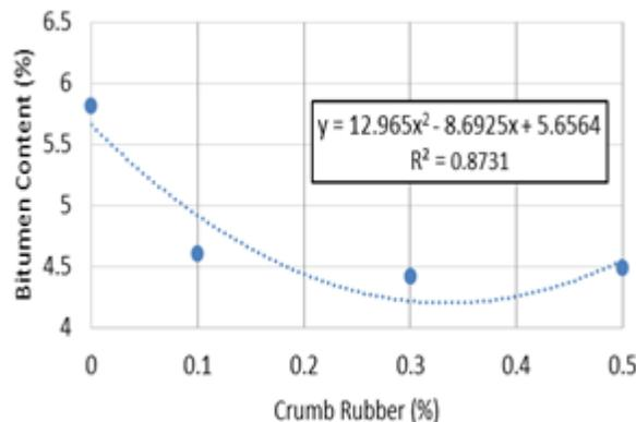
**Fig 5.** The Influenced of aggregate replacement by crumb rubber on the optimum bitumen content
