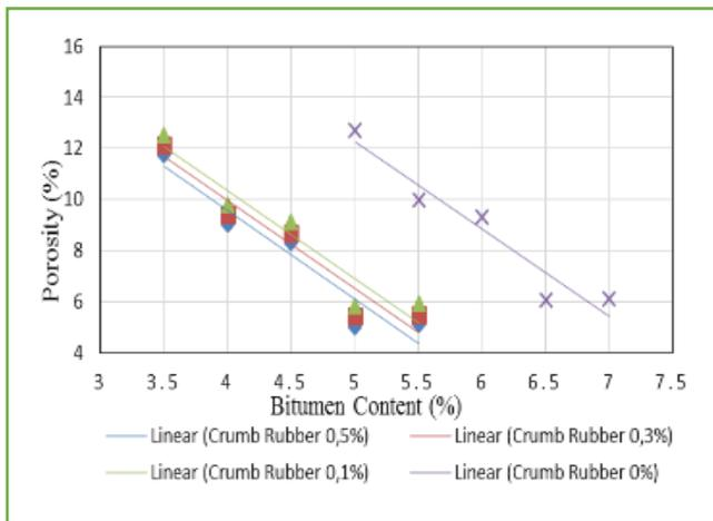
**Fig 4.** The porosity of thin surfacing hot mixture at various crumb rubber aggregate replacement
