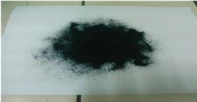
**Fig 3.** Crumb rubber as aggregate replacement made from waste recycled tires
