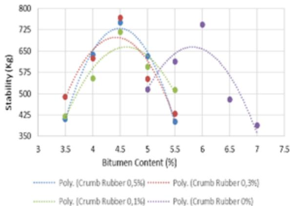
**Fig 3.** The stability of thin surface asphalt mixture at various bitumen and rubber contents
