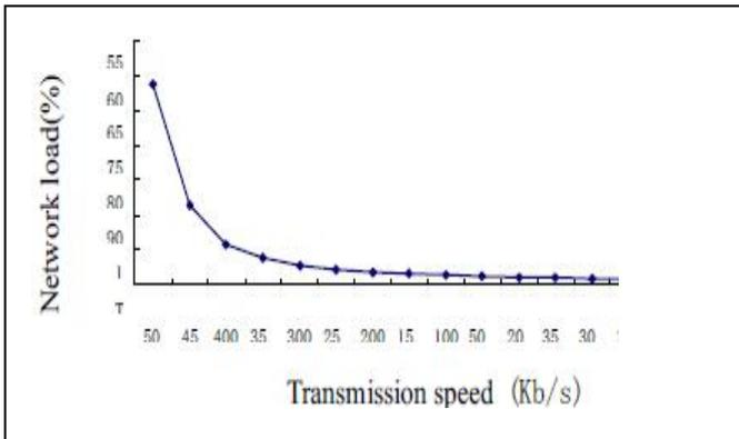
(Relation of CAN node's data transmission speed and network loads)
