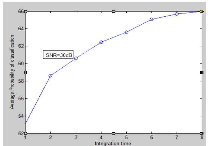
**Fig.9.** Classification rate of Cepstrum at 5 Feature vector at 30dB of SNR.
