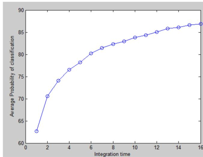
**Fig.10.**Classification rate of Bispectrum feature at 16 sec of integration time with 35 feature vector.
