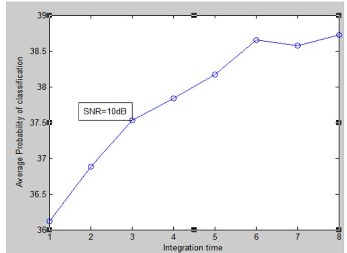
**Fig.7.** Classification rate of cepstrum at 5 Feature vector at 10dB of SNR.
