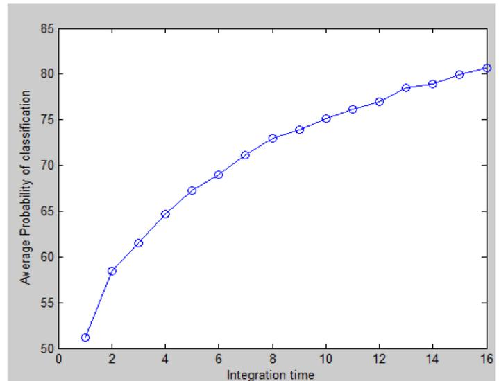
**Fig.11.**Classification rate of cepstrum feature at 16 sec of integration time with 35 feature vector. If we increase the feature vector size up to 50, then the classification results goes up to 90%.
