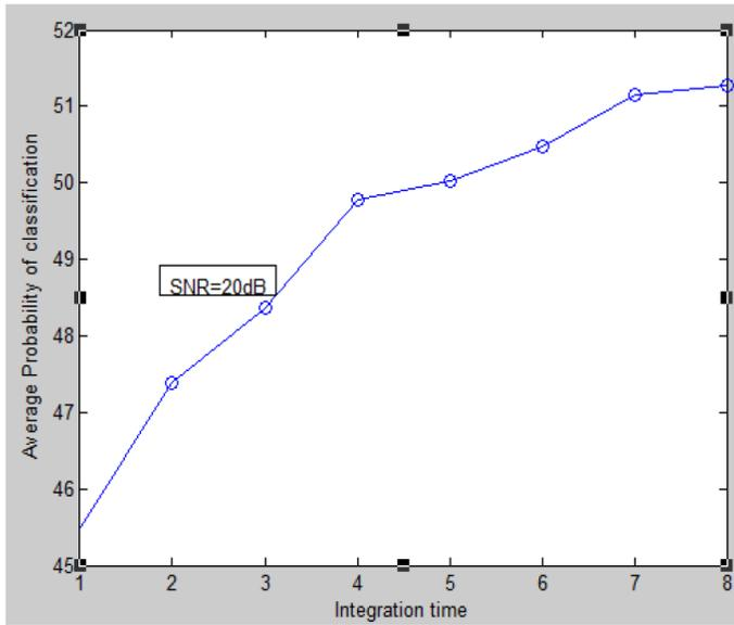
**Fig.5.** Classification rate of Bispectrum at 5 Feature vector at 20dB of SNR
