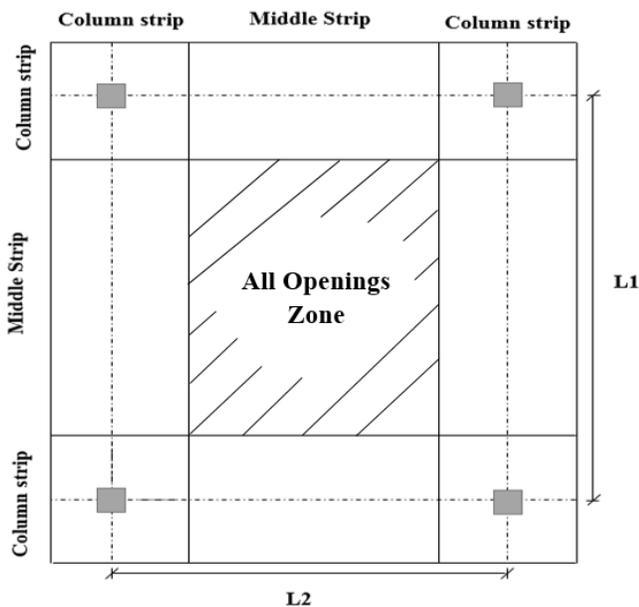
Figure (2) Location of opening in the two-way slab
