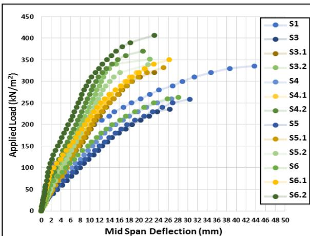
Figure (30) Load-deflection relationships at the mid span, for slab without openings (S1) and all slabs with two openings with and without strengthening
