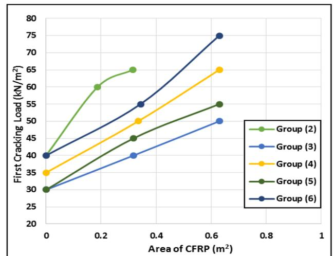
Figure (32) The effect of CFRP area on first cracking load
