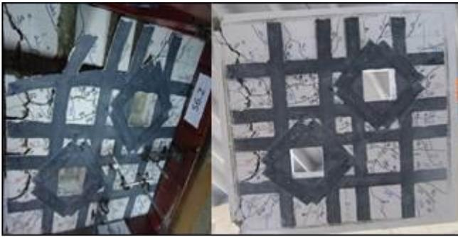
Figure (23) Cracks pattern after failure for slab S6.2
