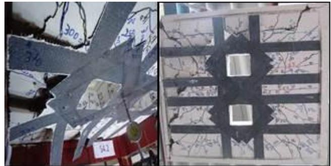
**Figure (17)** Cracks pattern after failure for slab S4.2
