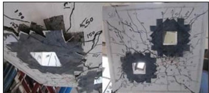
Figure (22) Cracks pattern after failure for slab S6.1
