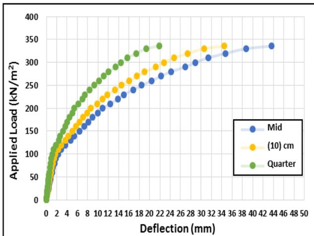
Figure (24) Load-deflection curve for group (1) (slab S1)
