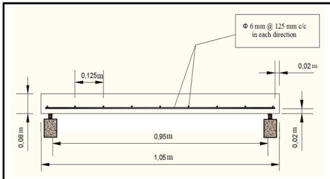
Figure (1) Details of reinforcement of the slab specimens
