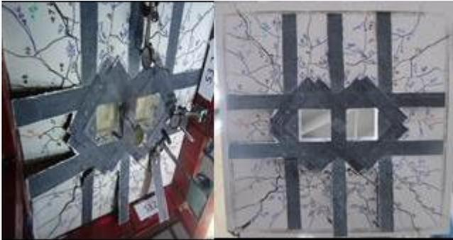
**Figure (14)** Cracks pattern after failure for slab S3.2
