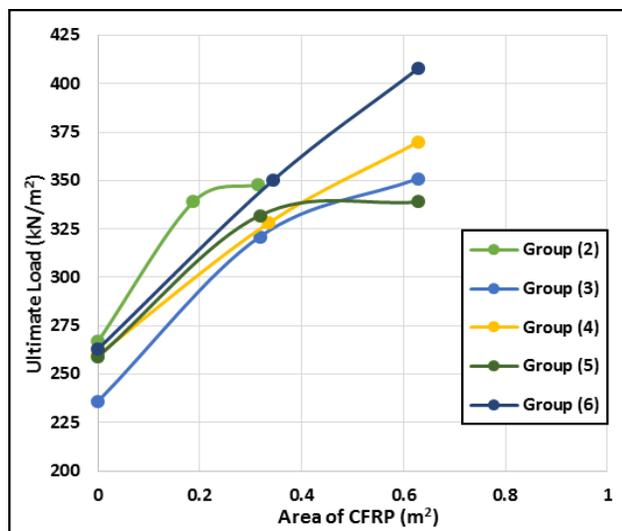
**Figure (33)** The effect of CFRP area on ultimate load
