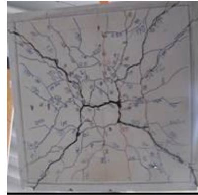
**Figure (8) Cracks pattern after failure for slab S1**
