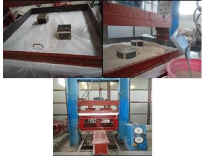
(7) Loading arrangement for uniform load test
