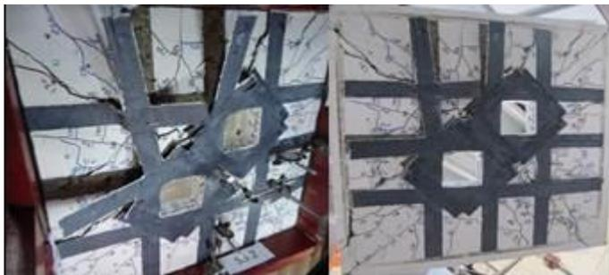
Figure (20) Cracks pattern after failure for slab S5.2
