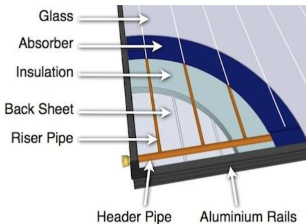
**Glass:** Toughened glass (glazing) protects the absorber from the outside environment while allowing through >90% of sunlight.
