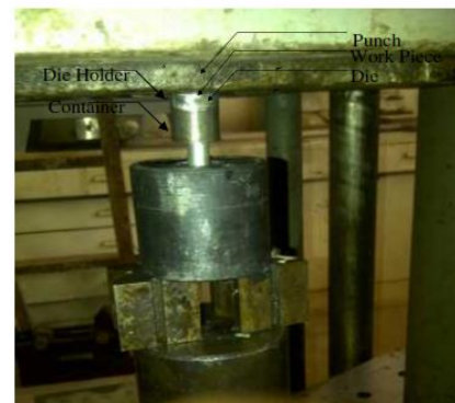
Figure 1: Extrusion die punch assembly on universal testing machine (UTM)
