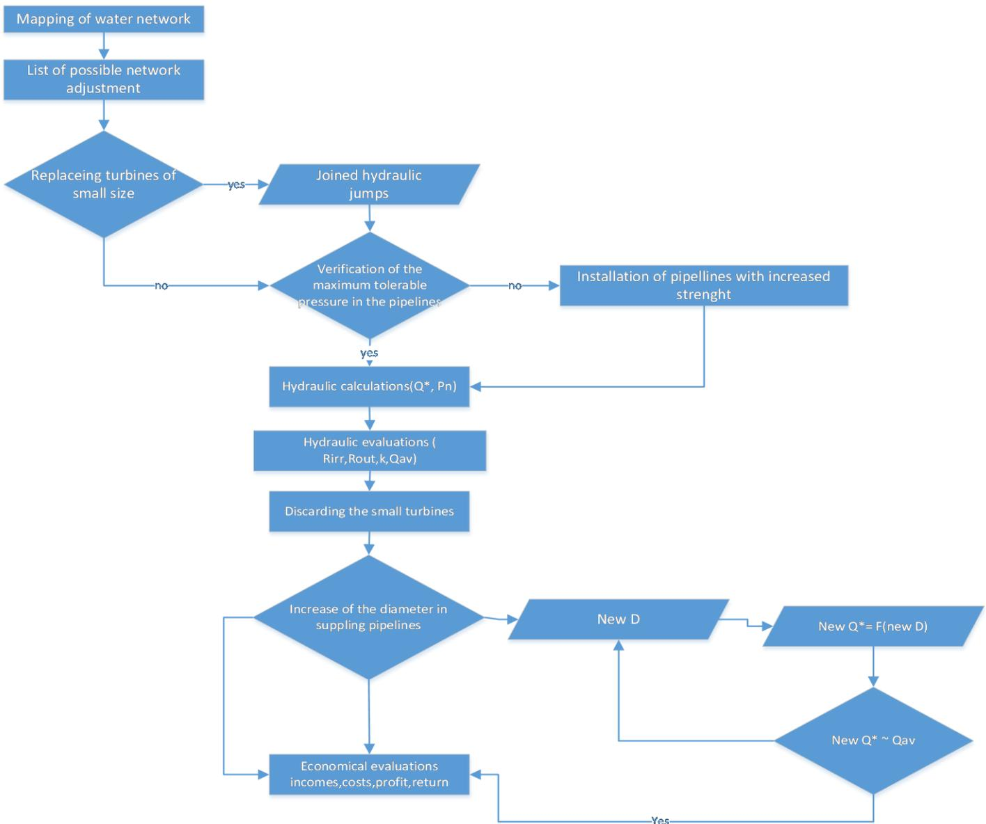
**Fig. 1.** Flow chart of the method for assessing MHP feasibility in existing irrigation systems.
