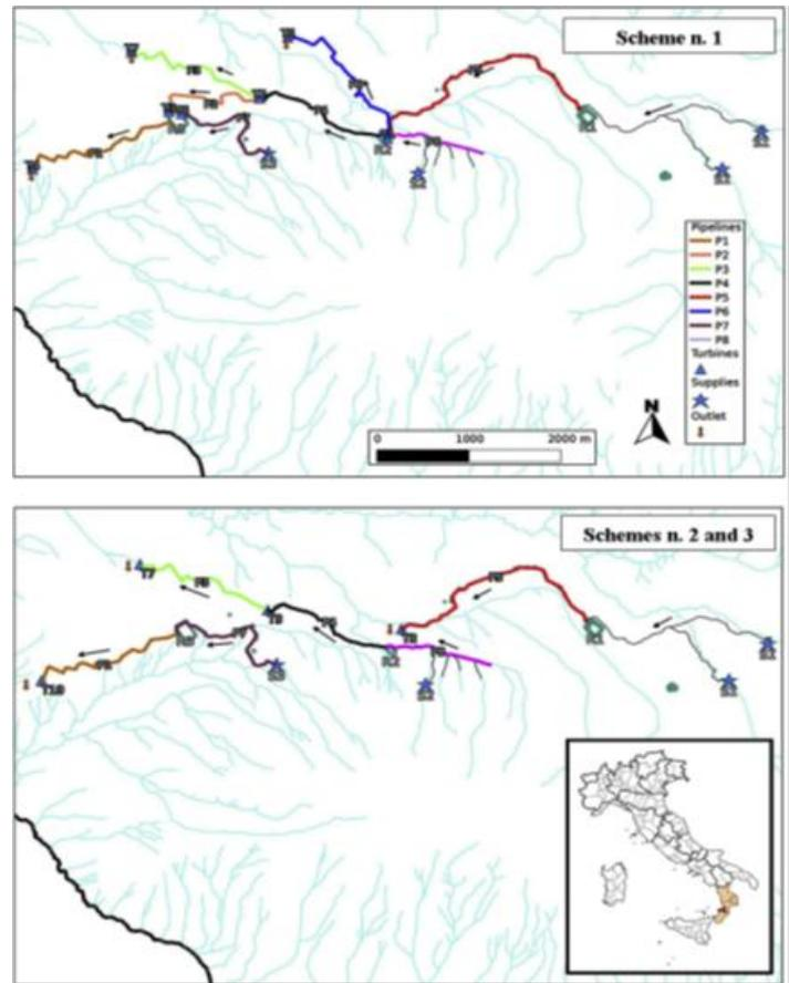
**Fig. 2.** Layout of three MHP outlines in the Spilinga-Ricadi irrigation system.
