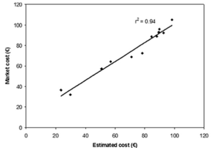
**Fig. 3.** Regression equation of CCEME of SHP plants in the Italian market versus those appraised by Equation (10) ( $b = \frac{1}{4}25635 V kW_{-0.7} m^{0.35}$ ).
