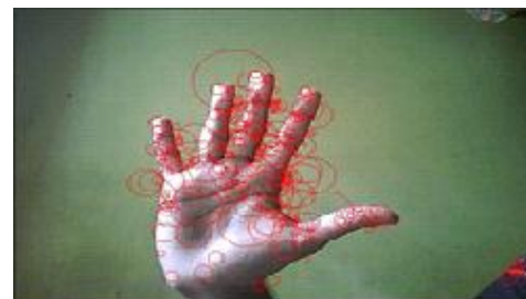
Figure 3. Example of SURF keypoints on a palm
