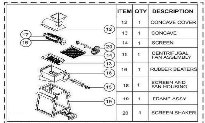
Fig. 1: Exploded view of the machine
