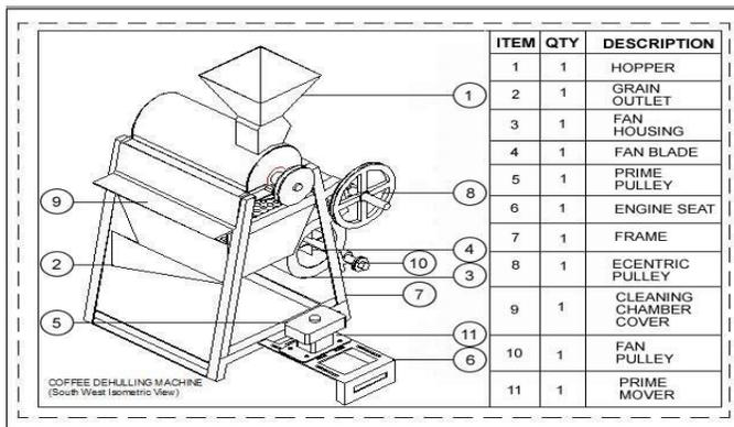
**Fig. 3: Isometric of the Hulling Machine**
