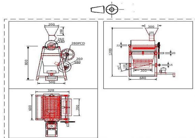
Fig. 2: Orthographic views of the machine
