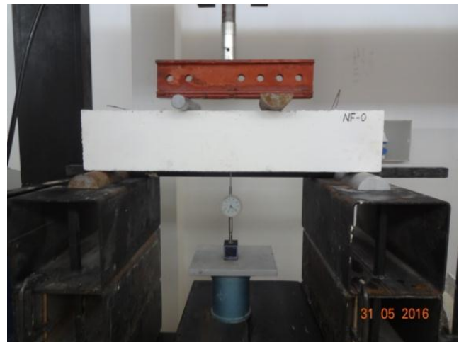
Fig. 1. TEST SET-UP ARRANGEMENT FOR BEAMS
