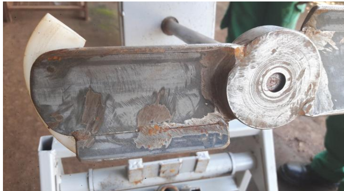
Figure 8: Banana juice extractor [Bottom view of the extraction impeller]. The materials used is neither food grade nor stainless steel. Corrosion is evident and a vast manifestation of crevices, poor surface finish and weldment.
