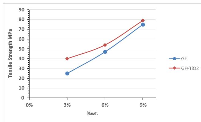
**Fig. 4** Effect short random glass fibers and titania particles on tensile strength of Epoxy
