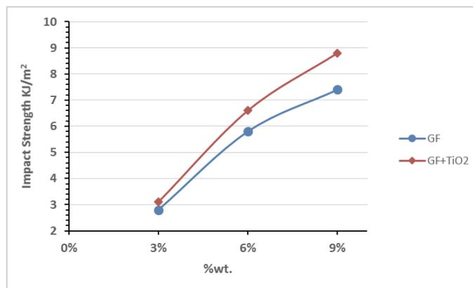
**Fig. 2** Effect short random glass fibers and titania particles on impact strength of Epoxy
