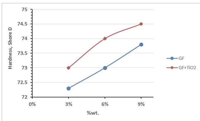
**Fig. 3** Effect short random glass fibers and titania particles on hardness of Epoxy
