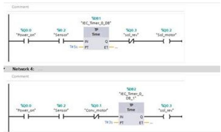
**Fig 10(b).** The Ladder diagram of the proposed system
