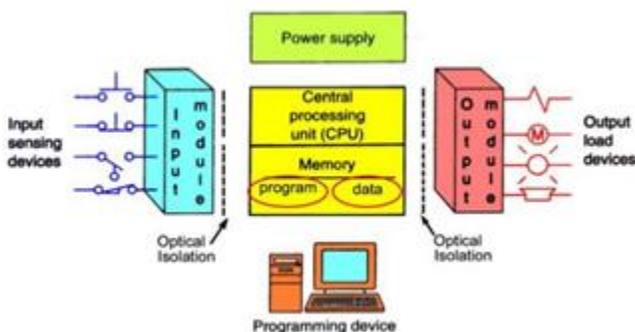
Fig 1. The Block Diagram of PLC System [4]
