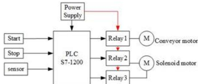
Fig 8. The Hardware Implementation of the proposed system
