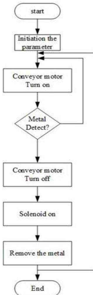
**Fig 9.** The flow chart of the proposed system
