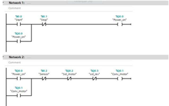
**Fig 10(a).** The Ladder diagram of the proposed system
