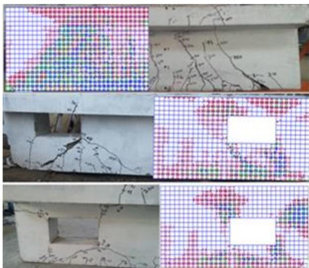
Figure (9) the experimental and predicted theoretical crack pattern of control specimens
