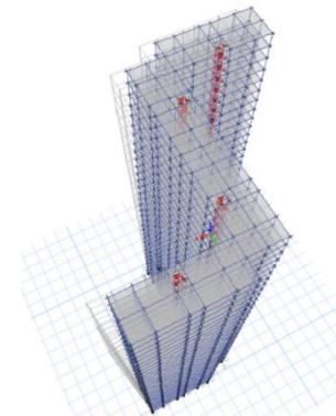
Fig. 3. 'S' Shape Deformed Structural Plan Model
