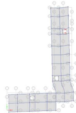
Fig. 3. 'L' Shape Deformed Structural Plan Model
