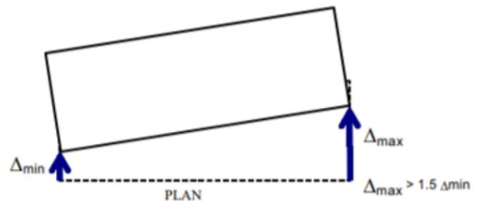
Fig. 1. Torsional Irregularity in Plan
