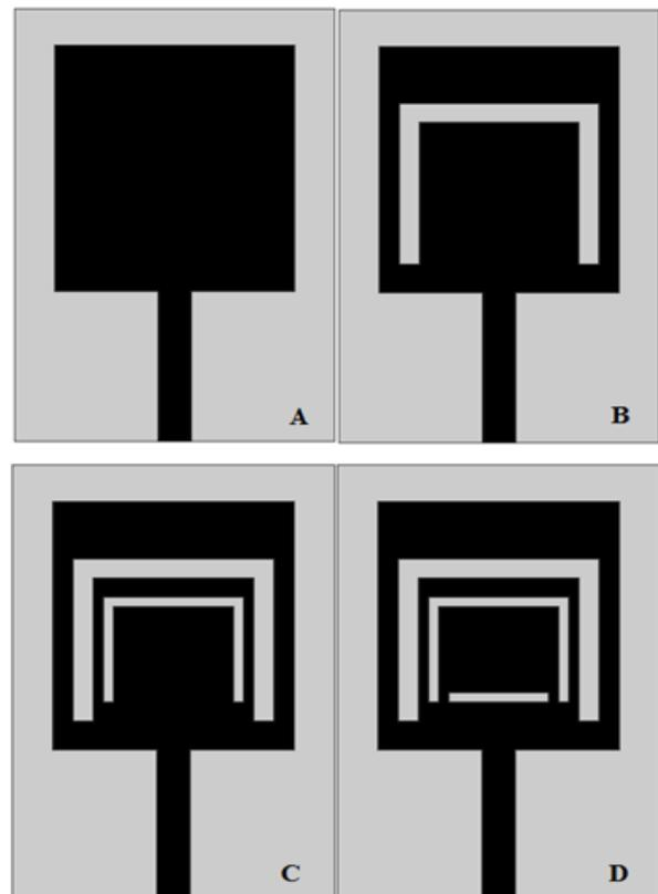
**Figure [1]** Design Steps of Proposed Antenna without Tuning Slot (A,B,C,D)
