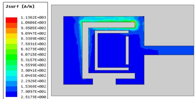
Figure [10] Current distribution in Proposed antenna
