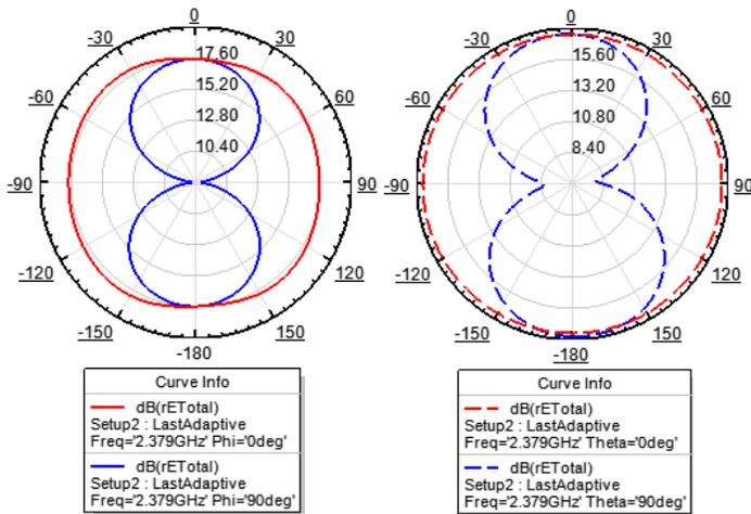
Figure [11] Radiation pattern curves in E and H plane for theta and Phi directions
