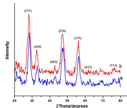
Fig.2: XRD pattern of CeNi<sub>0.5</sub>O<sub>y</sub> (a) and reduced CeNi<sub>0.5</sub>O<sub>y</sub> (b)
