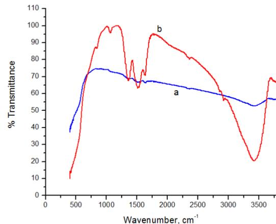
Fig.4: Transmittance spectra of  $\text{CeNi}_{0.5}\text{O}_y$  (a) and reduced  $\text{CeNi}_{0.5}\text{O}_y$  (b).
