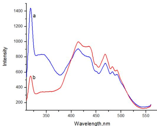
Fig.6: Emission spectrum of  $\text{CeNi}_{0.5}\text{O}_y$  (blue line) (a) and reduced  $\text{CeNi}_{0.5}\text{O}_y$  (red line) (b).
