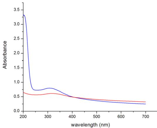
Fig.5: UV-Vis spectrum of (a)  $\text{CeNi}_{0.5}\text{O}_y$  (blue line) (b) reduced  $\text{CeNi}_{0.5}\text{O}_y$  (red line)
