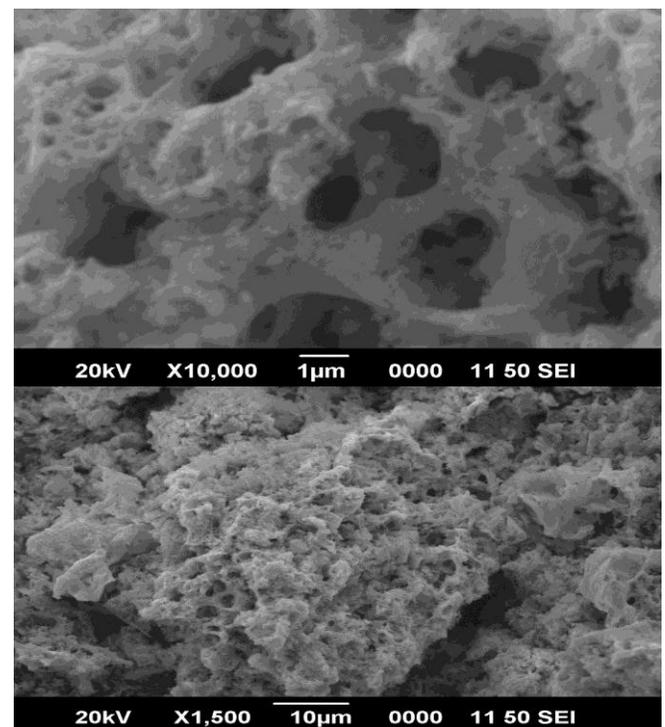
Fig.8: SEM images of  $\text{CeNi}_{0.5}\text{O}_y$ .
