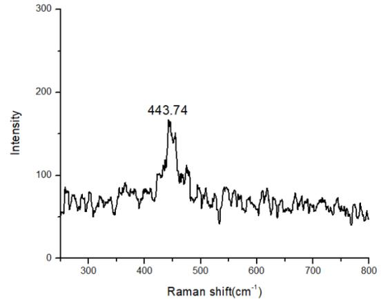
Fig.7: Raman spectrum of  $\text{CeNi}_{0.5}\text{O}_y$ .
