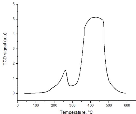
Fig.9: TPR spectra of H<sub>2</sub> adsorbed on CeNi<sub>0.5</sub>O<sub>y</sub>.
