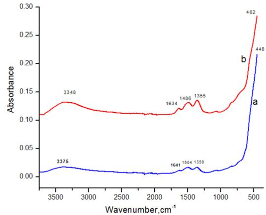
Fig.3: FT-IR spectra of  $\text{CeNi}_{0.5}\text{O}_y$  (a) and reduced  $\text{CeNi}_{0.5}\text{O}_y$  (b).
