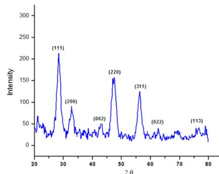
Fig.1: XRD pattern of CeNi<sub>0.5</sub>O<sub>y</sub>
