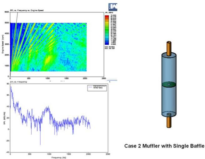
Case 2 Muffler with Single Baffle
