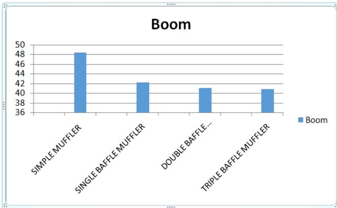
**Figure 13:** Comparison Bar chart for four cases of muffler with Rockwool as an absorptive material.
