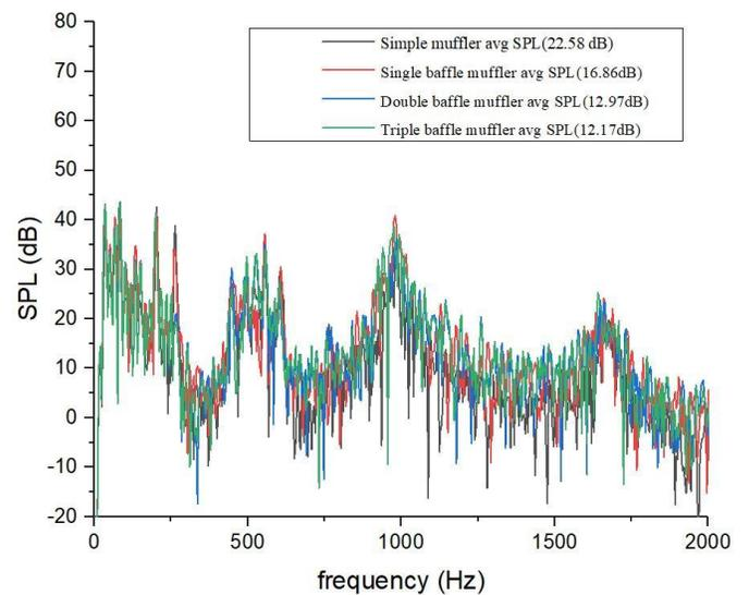
Figure 8: Comparison graph for four cases of muffler
