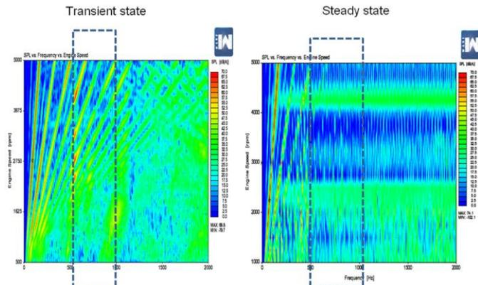
Figure 2: Colormap Representation for Transient and Steady State.
