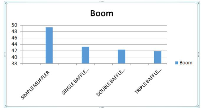
Figure 11: Comparison Bar chart for four cases of muffer with Glasswool as an absorptive material.
