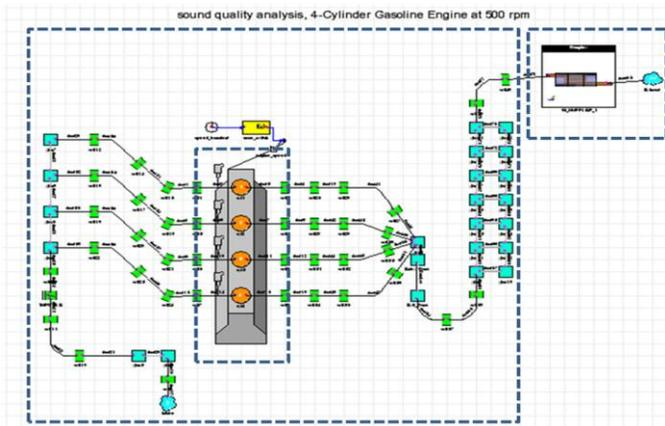
Figure 1: Ricardo Wave 1-D GUI for sound quality analysis.
