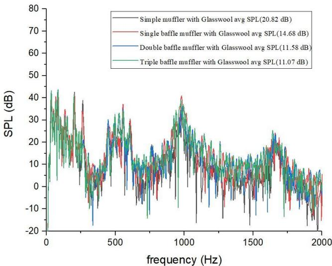
Figure 10: Comparison graph for four cases of muffer with Glasswool as an absorptive material.
