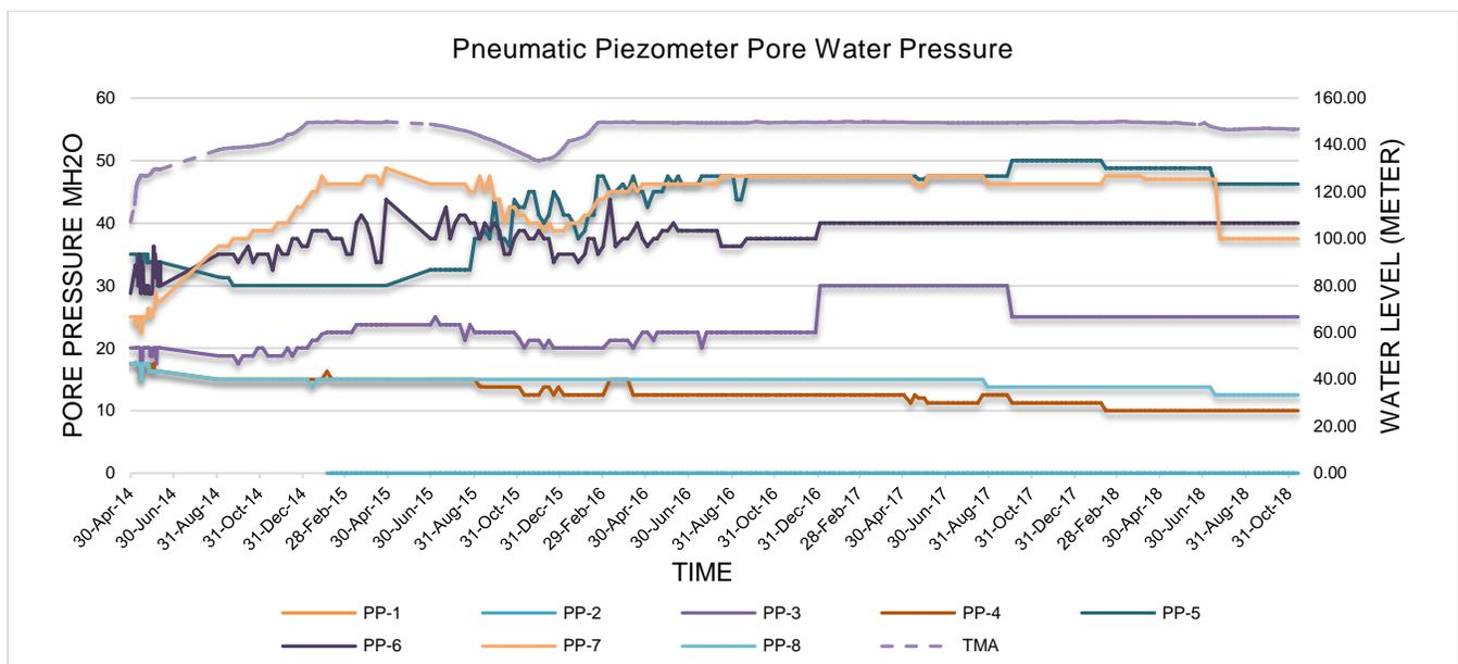
**Fig. 4** Graph of pore water pressure on the measured pneumatic piezometers
