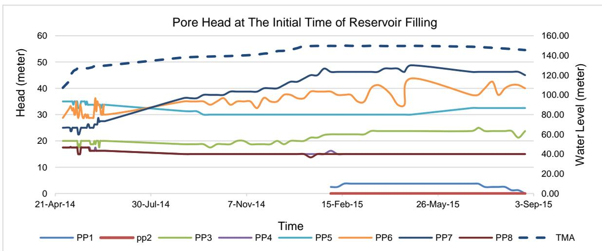
Fig.8 Correlation of pore water pressure with the reservoir water level
