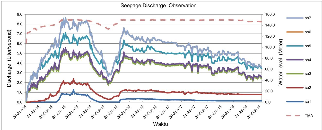
Fig. 5 Seepage graph on Seepage Observation
