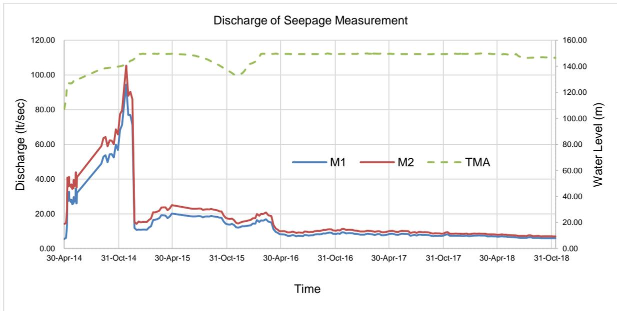
Fig.6 Graph of measured seepage on the dam's body
