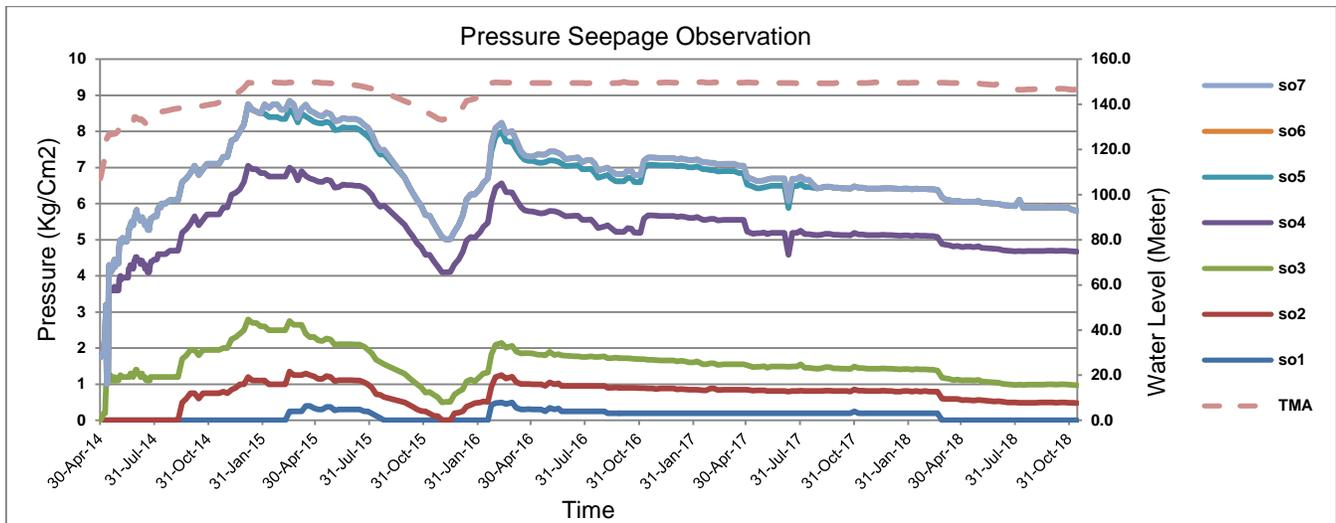
**Fig.3** Graph of Water Pressure on Seepage Observation
