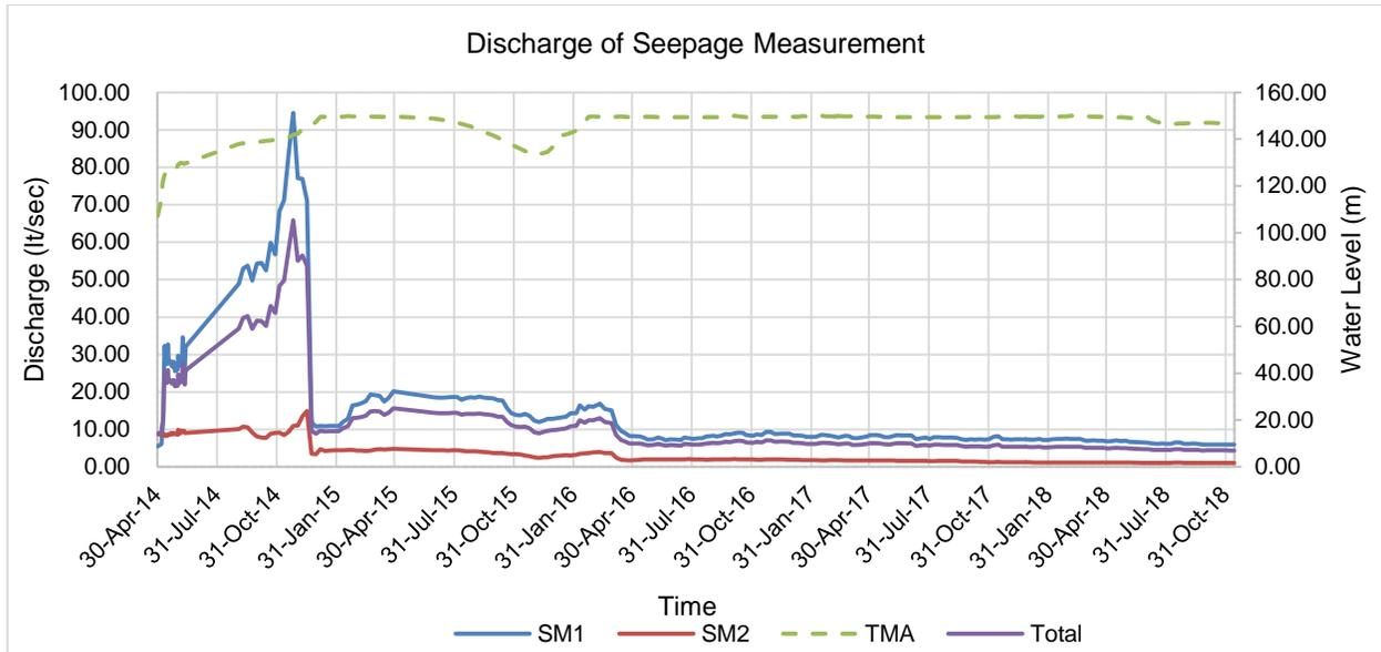
**Fig.9** Seepage graph (V-Notch) on the body of the Jatibarang dam
