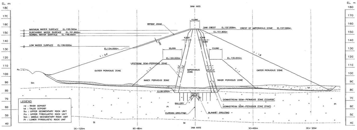
Fig. 1 Typical Section of Jatibarang Dam
