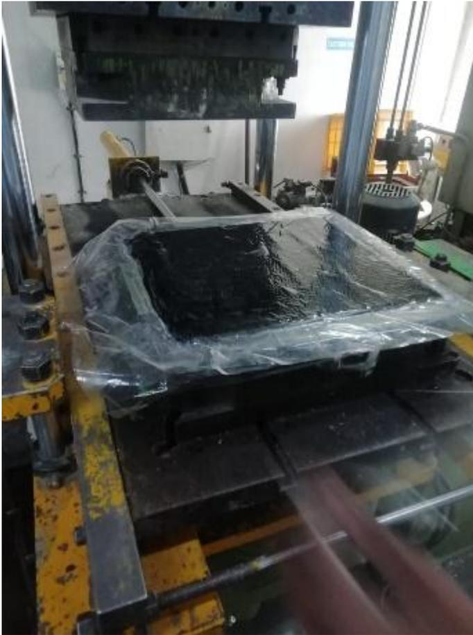
**Fig. 1.** Compression moulding of epoxy-carbon fiber sheet
