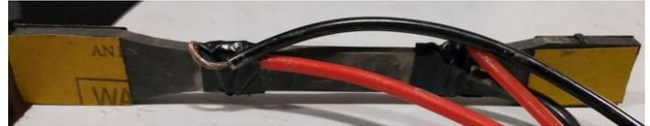
**Fig. 3.** Specimen of epoxy-carbon fiber composite
