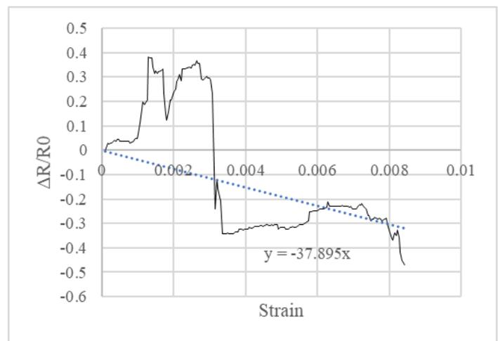
**Fig. 10  $\Delta R/R_0$  vs  $\epsilon$  (Slope shows GF)**
