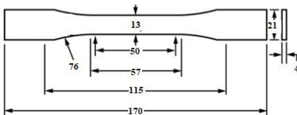
**Fig. 2.** ASTM D- 638 Specimen dimensions[9]
