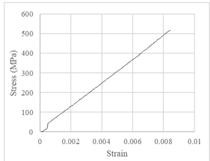
**Fig. 7.** Stress-strain curve obtained for unidirectional epoxy-carbon fiber composite. The peak stress before the cracking of the specimen was found to be 516.49 MPa.
