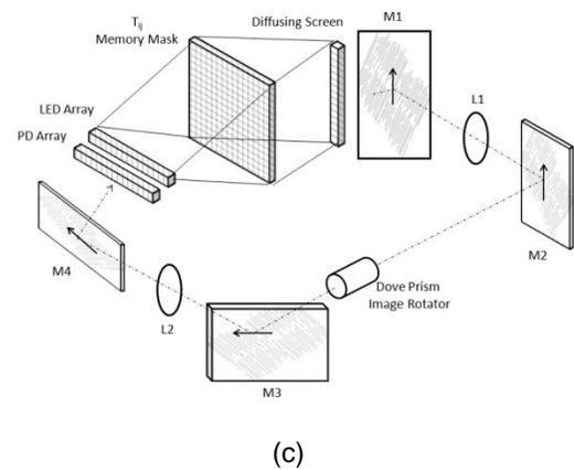
**Fig 1** Optical implementation of Hopfield Neural network (a) Matrix-vector multiplier incorporating non-linear feedback. (b) Realization of binary bipolar memory mask in incoherent light. (c) Optical feedback
