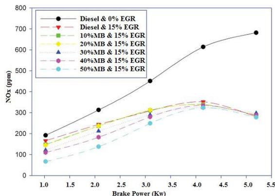
Figure.6 BP in KW vs NOx emission in ppm
