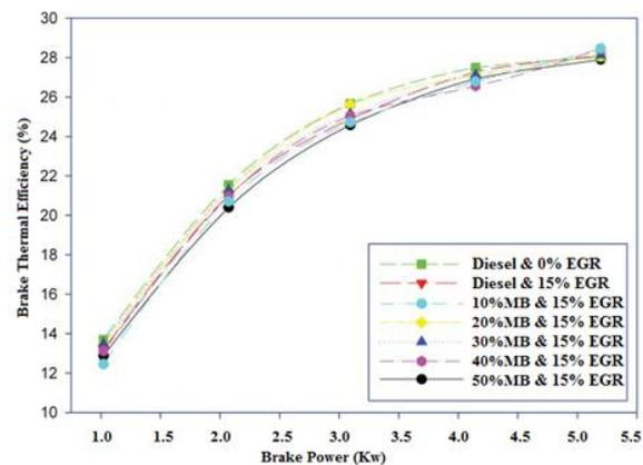
Figure.2. BP in kW vs BTE in %
