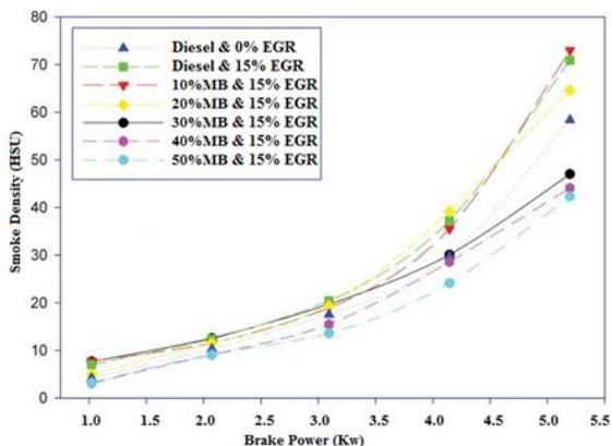
Figure.4 BP in kW vs smoke (HSU)
