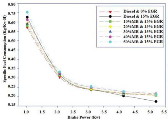
Figure.3. BP in kW vs Specific fuel consumption in kg/kWh
