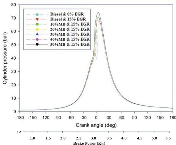
Figure.7. Crank Angle in degree Vs Cylinder Pressure in bar
