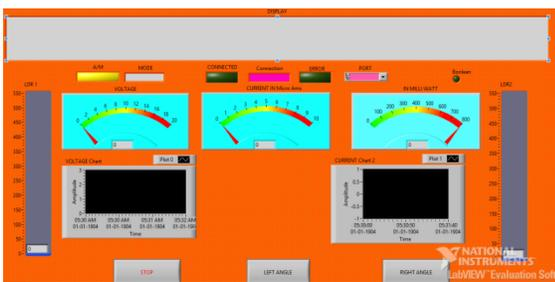
Fig.5. Front Panel in the LabVIEW
