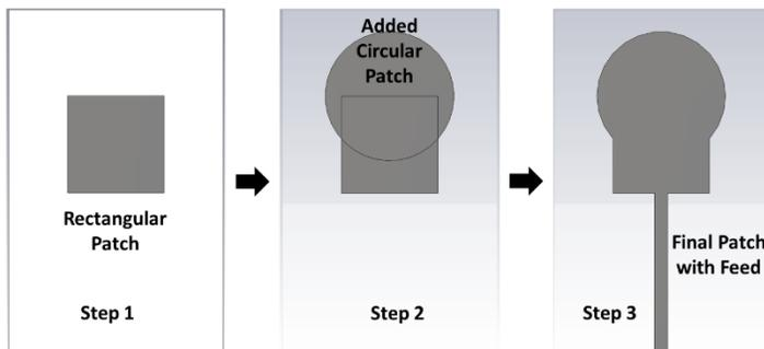
**Fig 2.** Steps of the antenna structure design
