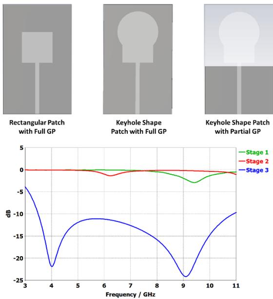
Fig 3. S-Parameter Response for different stages of design
