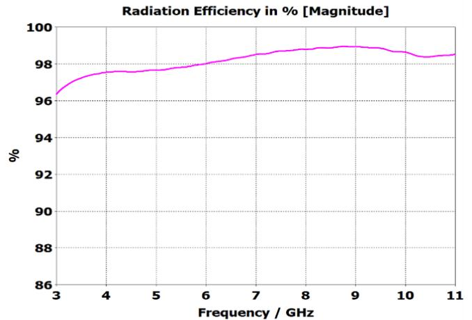
Fig 6. The radiation efficiency of the antenna
