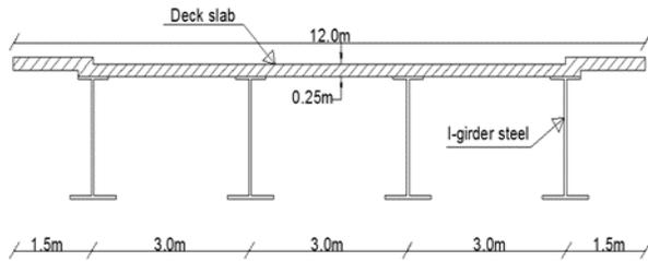
Fig. 4. Cross section of composite steel I-girder bridge
