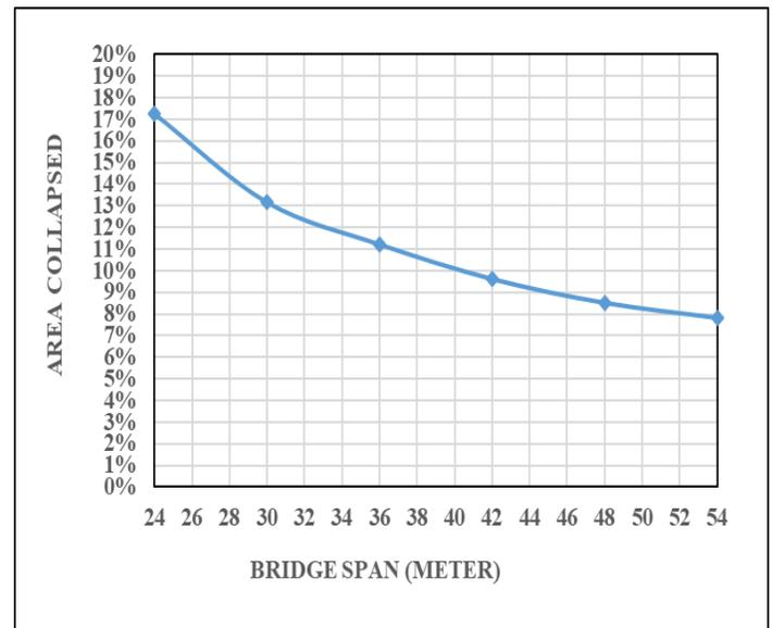
**Fig. 10.** Relationship between different bridge spans with percentage of area collapsed in reinforced concrete slabs
