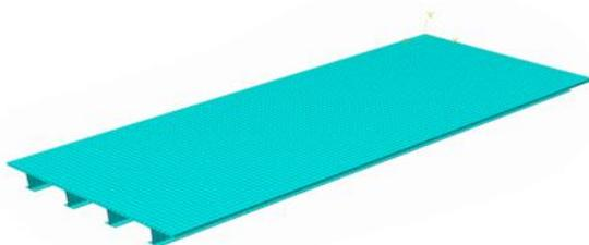
Fig. 6. Model of composite steel bridge using ABAQUS
