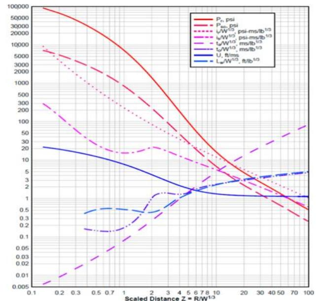
**Fig. 3. Positive phase shock wave parameters for explosion on free-air**
