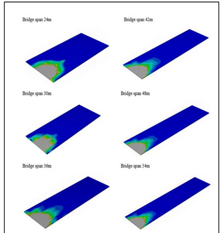
**Fig. 9.** Area collapsed in concrete slab at different bridge span
