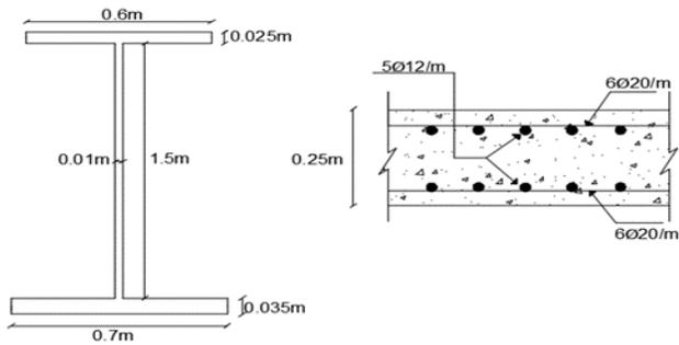
Fig. 5. Steel girders dimension and reinforcement of slab
