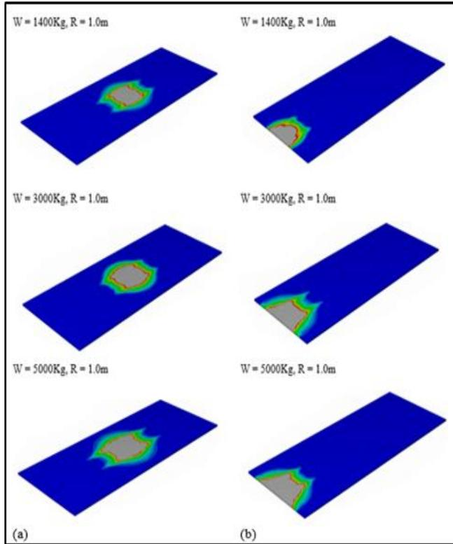
Fig. 7. Area collapsed in concrete slab at blast below the bridge (a) mid-span; (b) span end
