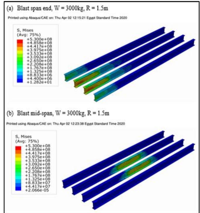
Fig. 8. Comparison between maximum stresses of steel girders at blast below the bridge
