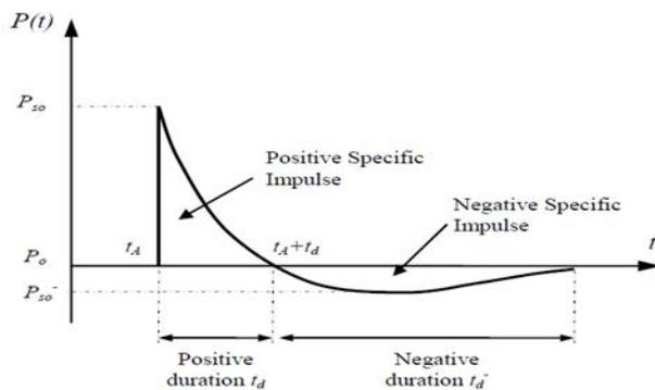
**Fig. 2. Typical the blast wave pressure-time profile**
