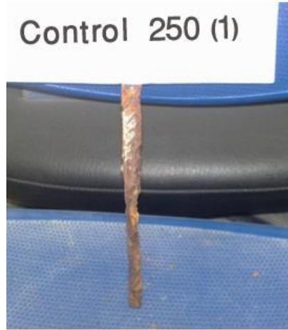
**Fig .5.** Bar after corrosion for Cylinder (C1)
