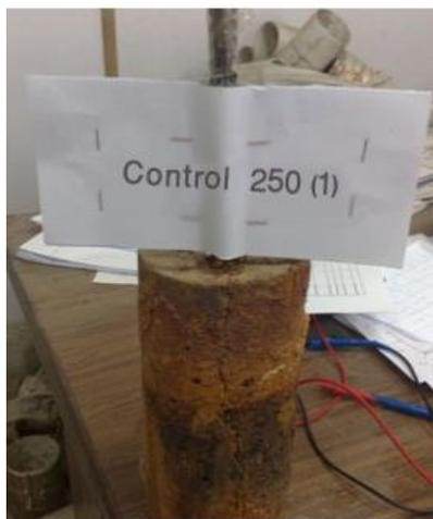
**Fig. 4.** Crack Pattern of Cylinder (C1)
