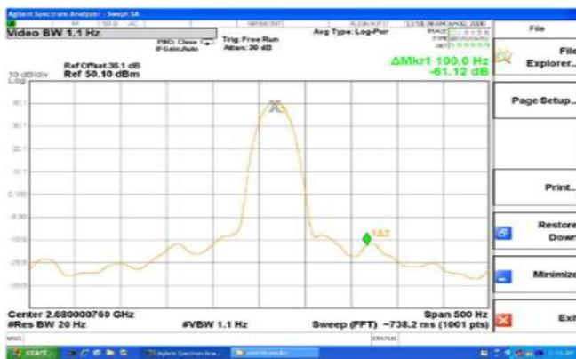
**Fig. 12(a): Phase Noise at 100Hz offset**
