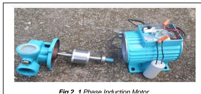
Fig 2 1 Phase Induction Motor
