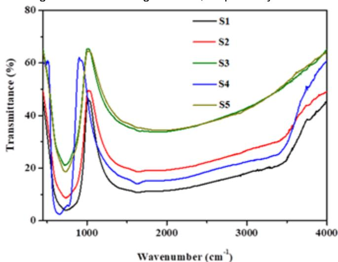
**Fig. 2. IR spectra of (89.6-x)TeO<sub>2</sub>-10MgO-xSm<sub>2</sub>O<sub>3</sub>-0.4AgCl glass system**
