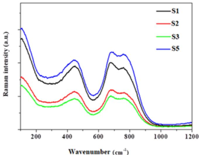
**Fig. 3. Raman spectra of  $(89.6-x)\text{TeO}_2-10\text{MgO}-x\text{Sm}_2\text{O}_3-0.4\text{AgCl}$  glass system**
