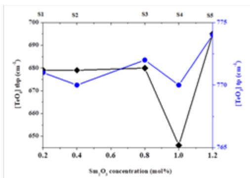
Fig. 4. The wavenumber of TeO<sub>4</sub> tbp and TeO<sub>3</sub> tp versus Sm<sub>2</sub>O<sub>3</sub> concentration
