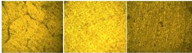
Fig. 10. Optical micrographs of the (a) original cast microstructure of pure Al, and after FSP with a 189 mm min -1 travel speed and 710 RPM rotation rate, from (b) the advancing edge and (c) retreating side, at mid-depth of the PZ.
