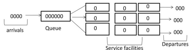
**Figure 4: Multiple-servers, Multiple-phase System**
