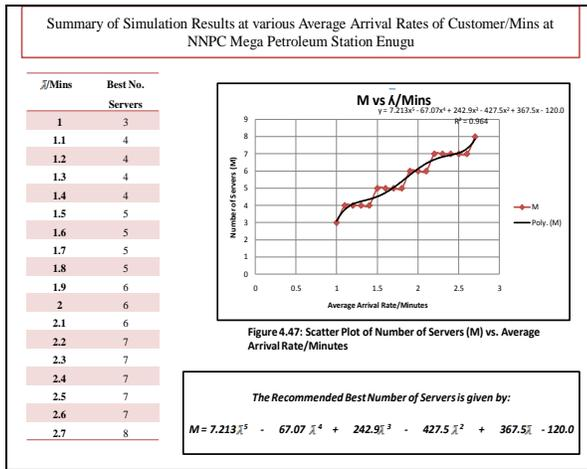
Figure 7: Summary of Simulation Results at various Average Arrival Rates of Customer/Mins at NNPC Mega Petroleum Station Enugu
