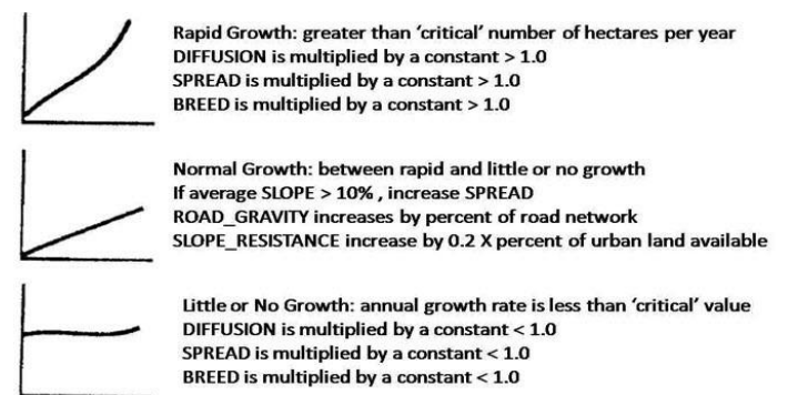
Figure 3: Self-modification adjustments to the control parameters
