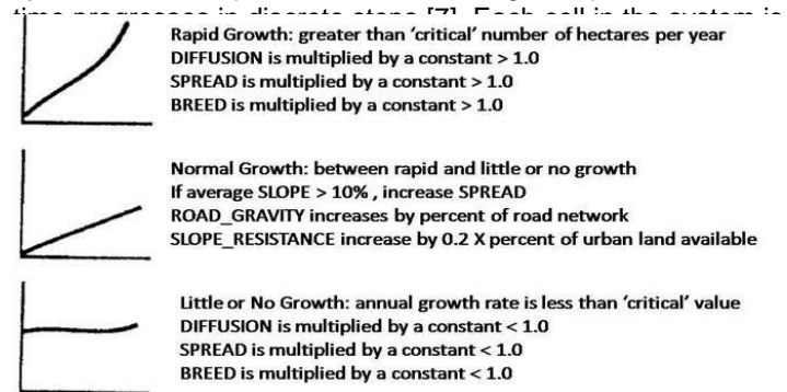
Figure 3: Self-modification adjustments to the control parameters
